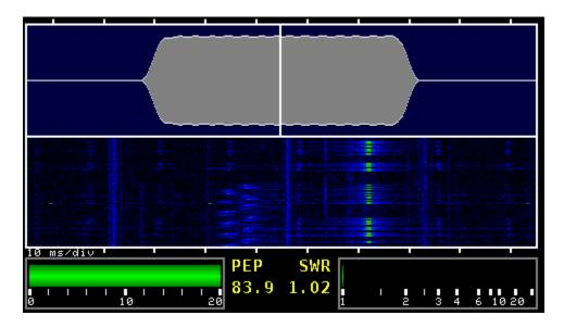
The display can also be set up to display a longer scale and monitoring high-speed CW elements ( $\sim$  50 wpm).
