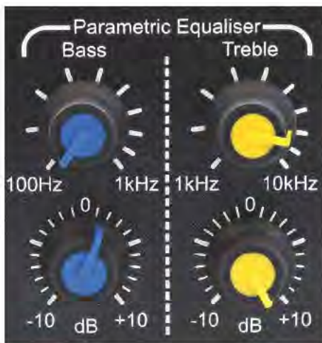
PHOTO 3: Close-up view of the filter control panel.
